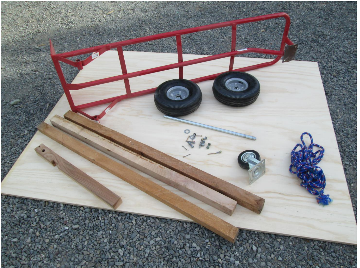
Prior to the activity weld on the mounting plate for the castor to the hand cart handle, and have plenty of odds n ends of timber to be used to join the plywood pieces
