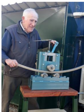
Ring roller made at the shed
