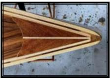
The construction is cedar strips, then covered with fibreglass inside and out to create the very strong waterproof hull and finished with UV resistance marine varnish.
