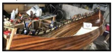
Much sanding was required, using progressively finer paper, to finally end with 400 grit wet sand. After vacuuming out the garage I lined the room with plastic film to create a 'dust free' paint booth before applying three coats of marine varnish.
