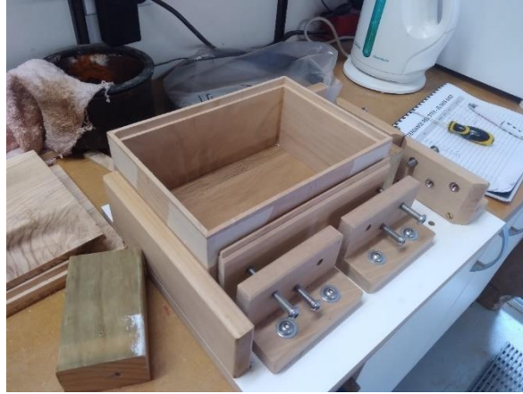
Box in glue up jig. This makes sure it is nice and square
